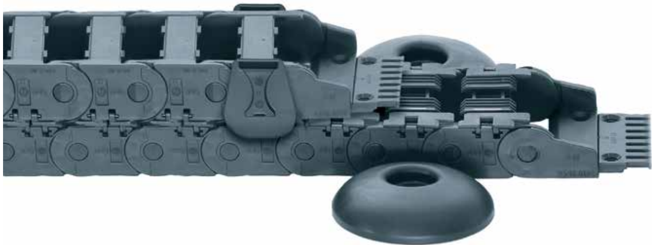
Series 2600AG - snap-open along the inner radius - crossbars with molded-on autoglide grooves
