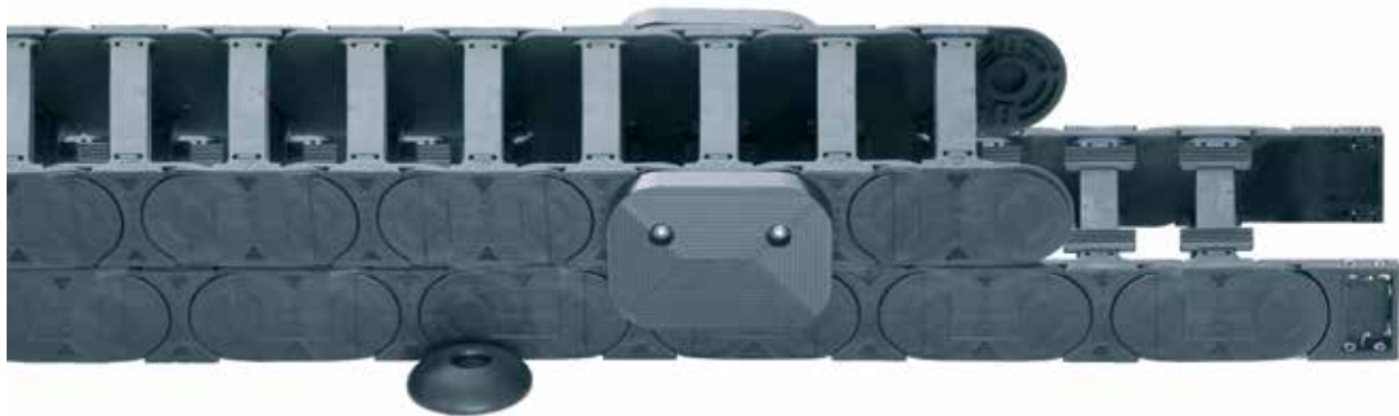
Series E4-42AG - openable along both radii, crossbars every link - autoglide crossbars along the inner radius
