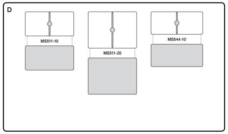
**ATTENTION!** Do not attempt to assemble snap cover on frame prior to PCB assembly. Covers are difficult to remove from non-soldered frames.
