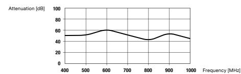
[Typical performance of 51.1mm x 38.4mm EMI/RFI shield as reference]
