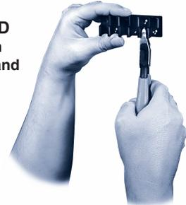
2. Cut the multiple tubing holder at a desired position and mount it on the equipment with the attached phillips countersunk tapping screws.
