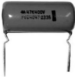
The Type PVC is a sturdy film and extended foil construction ideal for bypass and coupling applications. Extended foil construction is as good as it gets for low DF and high current applications. The PVC is encapsulated in a rugged, flame retardant, epoxy coating with the leads crimped to provide secure seating on printed circuit boards.
