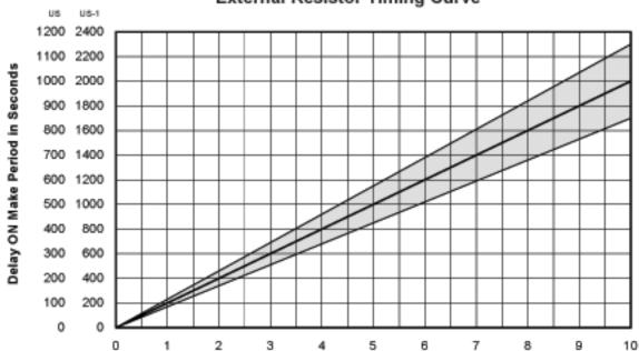
Value of External Resistor in Meg Ohms 1 Meg Ohm = 1,000,000 Ohms
