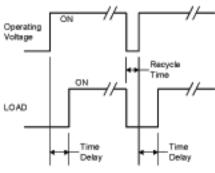
Load turns ON after time delay, remove power for Recycle Time to reset timer
