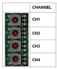
To modify the output voltage of each channel, operate on the R202 (for CH1), R204 (CH2), R206 (CH3) and R208 (CH4).
