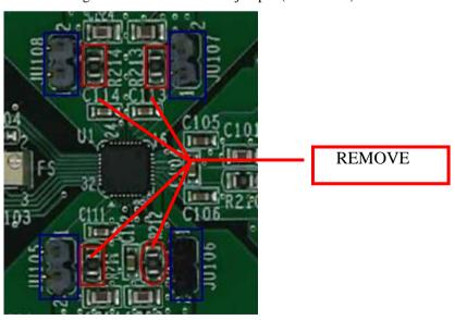
If a voltmeter is preferred, the  $0\Omega$  resistors need to be removed and a 0805 shunt need to be inserted; the following shunt values are suggested:
