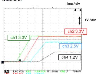
**NOTE:** The ON threshold (Vth) for SHDNBx pins can be anywhere between 0.8V and 2V so, in order to define the voltage at which the channel will be turn on, a voltage divider must be implemented, taking in account that SHDNBx pins have an internal  $400k\Omega$  pull-down resistor. As safety rule, Please make sure that input voltage divided by external resistor on SHDNB pins shall not be lower than 1.4V.
