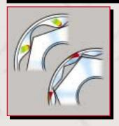
The Metrinch Wall Drive Profile was designed to provide a greater area of force application, compared with that applied by conventional tools. This profile, because of the buttress effect of its load bearing lugs, does not transmit the extreme peaks found when a tool with a wedge shaped profile is used. In distributing the torque load to the fastener trough the flats, the Metrinch tool does not only achieve greater force, but also lowers the
