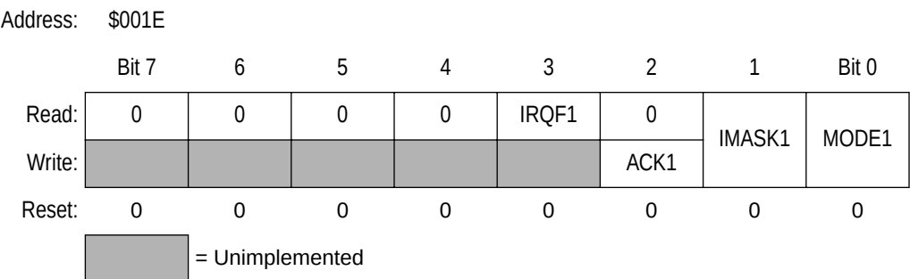
Figure 13-3. IRQ Status and Control Register (ISCR)
